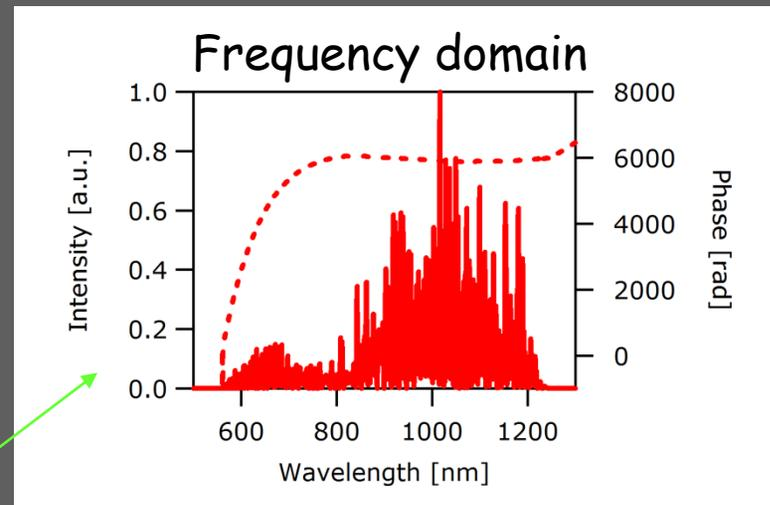
The XFROG-measured spectrum contains much more structure than the spectrum-measured with a spectrometer.
