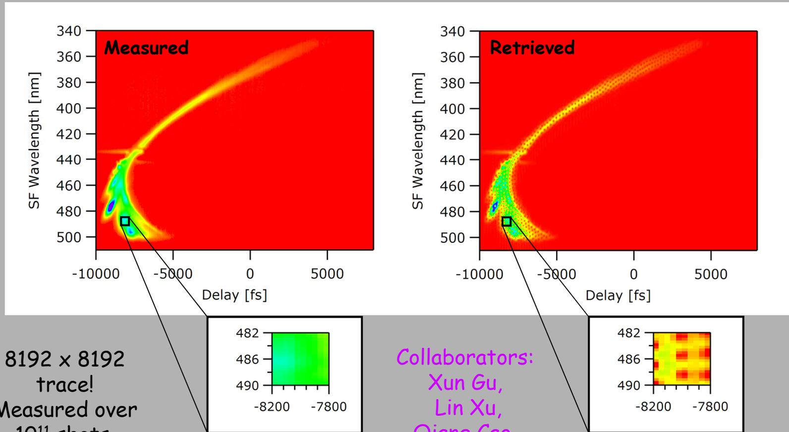
While the large-scale structure of each trace is identical, the measured trace lacks the fine-scale structure of the retrieved trace.
