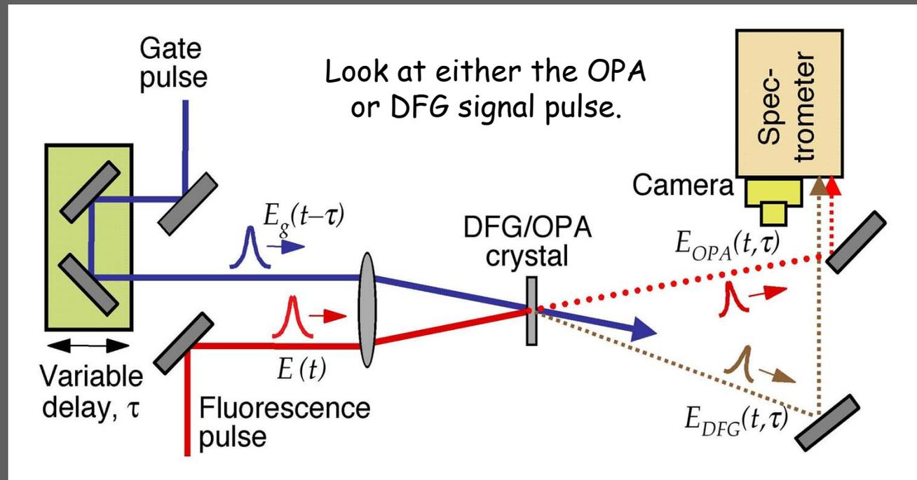
Absolute phase and spatial coherence don't affect FROG measurements. We must, however, modify the FROG algorithm for these processes: the gate function is now:  $\exp[g|E_{\text{gate}}(t)|]$ . But this is easy.
