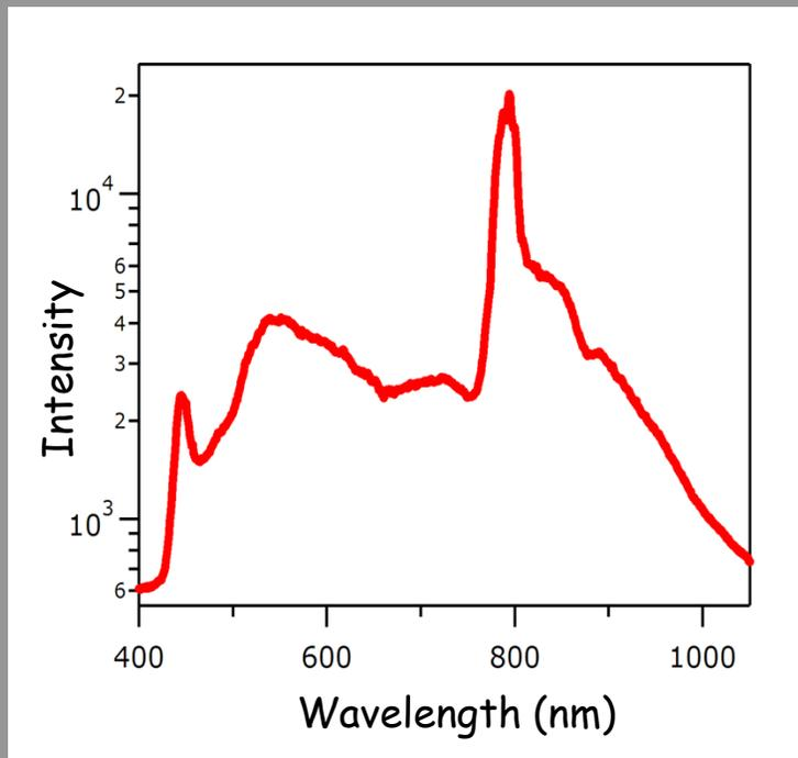
A typical microstructure-fiber continuum spectrum generated in our lab by a train of 30-fs Ti:Sapphire oscillator pulses.
