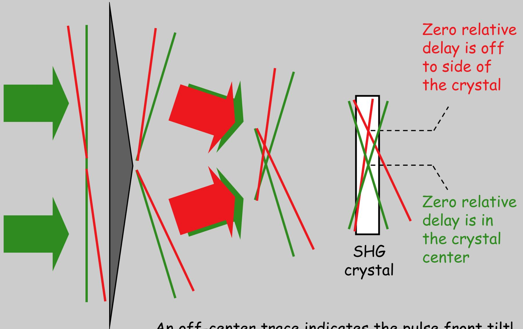
An off-center trace indicates the pulse front tilt!
