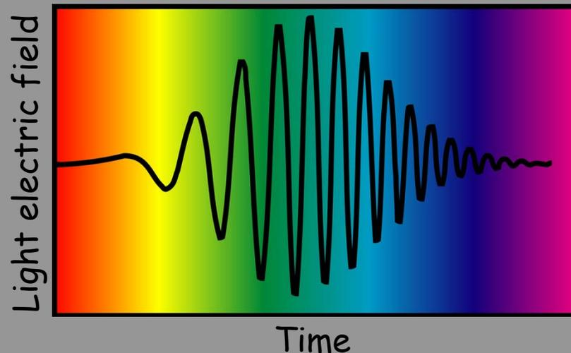
We'd like to be able to measure, not only linearly chirped pulses, but also pulses with arbitrarily complex phases and frequencies vs. time.
