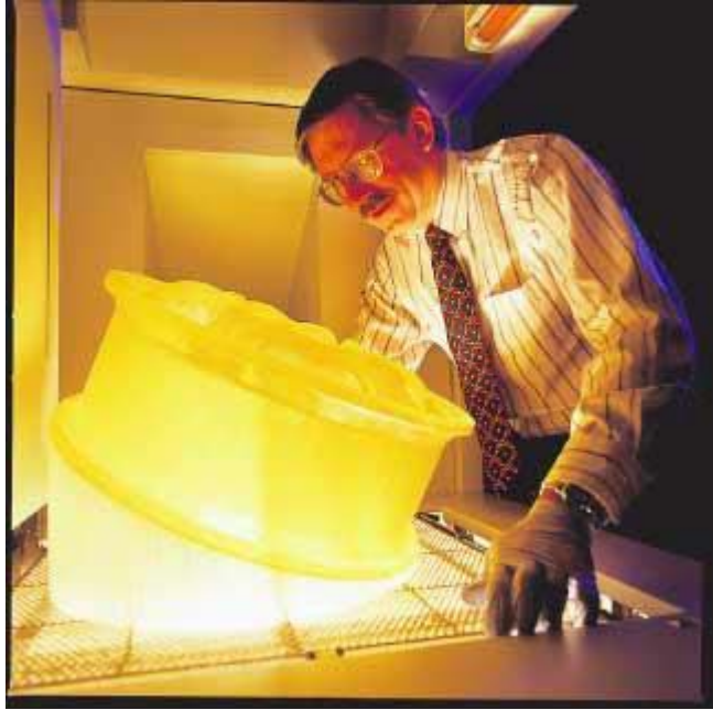
FIGURE 1. Rapid prototyping forms plastic models from CAD/CAM designs in a matter of hours. This system uses the 355-nm third harmonic of a Nd:YLF laser that delivers 800 mW to the surface of the epoxy vat.
